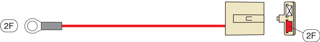
“EE” GM “SI” Alternator Exciter Wiring
